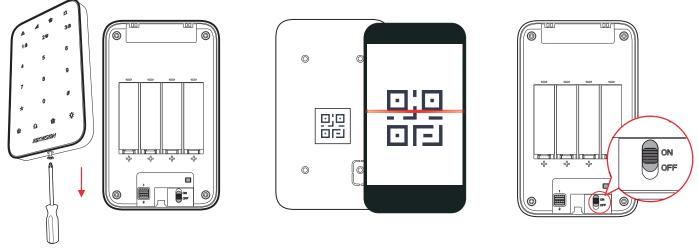
Scan the QR code on the rear panel of the keypad. Push the power switch to ON. Remove the screw on the bottom of the keypad. Disassemble the keypad and remove the rear panel.
